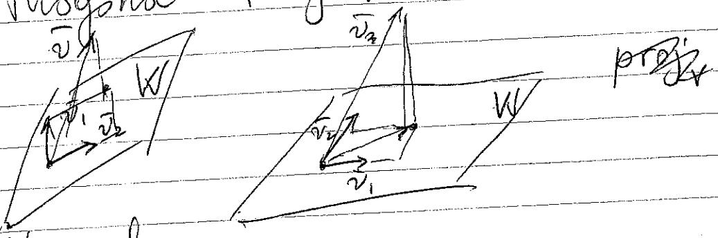
orthogonal projection of  $\bar{v}$  to  $W$  is  $\text{proj}_W \bar{v} = c_1 \bar{v}_1 + c_2 \bar{v}_2$
