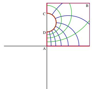
Only the first quadrant is shown. The part containing fluid is marked in red. The free streamline about the vortex is drawn as circular, although we will see that it is not, but all that matters here is that the z picture should give an idea of the flow. It is the  $\zeta$  and W pictures which need to be accurate.
