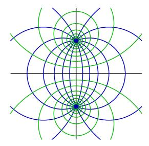
The branch cut in the logarithm, corresponding to rays beginning at the vortices and extending away from the centre of symmetry, isn't physically significant. Because there are closed streamlines there is no way to define a single-valued velocity potential everywhere. We could
