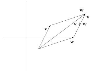
The triangles you would make for  $\mathbf{v} + \mathbf{w}$  and for  $\mathbf{w} + \mathbf{v}$  will form a parallelogram if you start them at the same point. And the sum of the two vectors appears as the diagonal of a parallelogram (the diagonal from the starting point).
