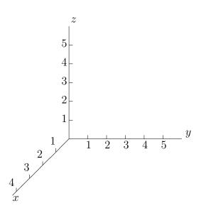
You can see we need to imagine the x-axis as coming out of the picture towards us. And we have a scale on each axis.
