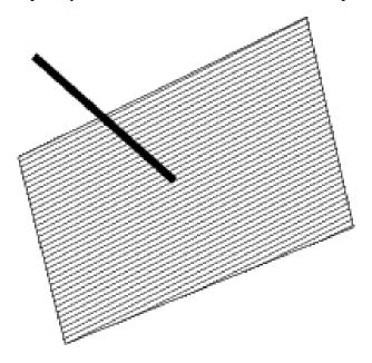
You should see that picking a vector perpendicular to it allows you to say which way a plane is tilted in space. The normal vector is not unique — multiplying the vector by a positive or negative (but not zero) scalar will not change the orientation of a perpendicular plane.
