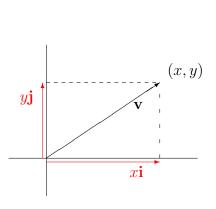
To check this look at the right-angled triangle with the vector along the hypoteneuse, horizontal side of length |x| and vertical side of length |y|.
