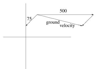
The resultant ground velocity (speed and direction) will be somewhat more to the SouthEast than due East and have a magnitude smaller than 500.
