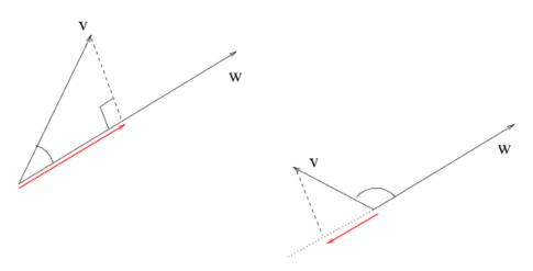
The 'length' of the projection will be  $\|\mathbf{v}\| \cos \theta$  where  $\theta$  is the angle between the two vectors. At least that is the length in the case when the angle  $\theta$  is an acute angle.
