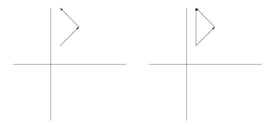
Because the two displacements make a right angle with each other, we can easily work out a precise answer. You would end up due North of where you started, and a distance  $\sqrt{2}$  away from the start.
