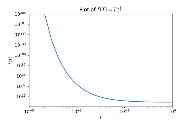
Since  $S = \frac{3N\hbar\omega_E}{Te^{\frac{\hbar\omega_E}{k_BT}}} = \frac{3Nk_B}{f\left(\frac{k_BT}{\hbar\omega_E}\right)}$  is simply a scaling of  $\frac{1}{f(T)}$  and T, we can deduce that S must also be 0 for small T, i.e.
