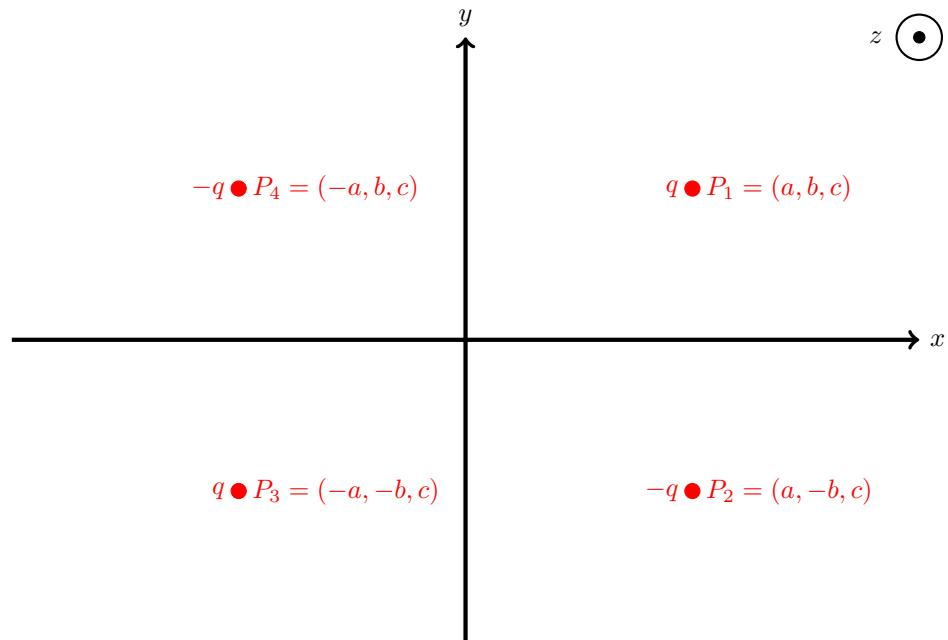
$$\begin{aligned}\Phi(\vec{r}) &= \frac{1}{4\pi\epsilon_0} \left( \frac{q}{|\vec{r} - \vec{P}_1|} + \frac{-q}{|\vec{r} - \vec{P}_2|} + \frac{q}{|\vec{r} - \vec{P}_3|} + \frac{-q}{|\vec{r} - \vec{P}_4|} \right) \\ &= \frac{q}{4\pi\epsilon_0} \left( \frac{1}{r_1} - \frac{1}{r_2} + \frac{1}{r_3} - \frac{1}{r_4} \right)\end{aligned}$$
