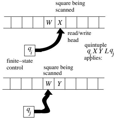
One thinks of the Turing machine as having memory, in the form of a ‘paper’ tape, a *finite-state control*, which can ‘adopt’ one of finitely many ‘states,’ and a *read/write head* which is positioned at a tape square, and can move to the next square on the left or right.
