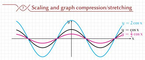
Let s denote the scaling function, s(x) = cx. Replacing a function f(x) by  $cf(x) = (s \circ f)(x)$  stretches the graph vertically if c > 1, and compresses the graph vertically if 0 < c < 1.
