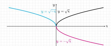
Let r denote the reflection function, r(x) = -x. Replacing a function f(x) by  $f(-x) = (f \circ r)(x)$  reflects the graph about the y-axis, and replacing f(x) by  $-f(x) = (r \circ f)(x)$  reflects the graph about the x-axis.
