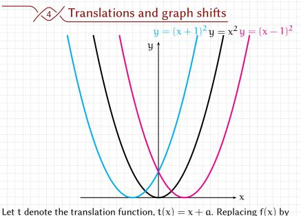
Let t denote the translation function, t(x) = x + a. Replacing f(x) by  $f(x + a) = (f \circ t)(x)$  shifts the graph horizontally: left if a > 0, right if a < 0.
