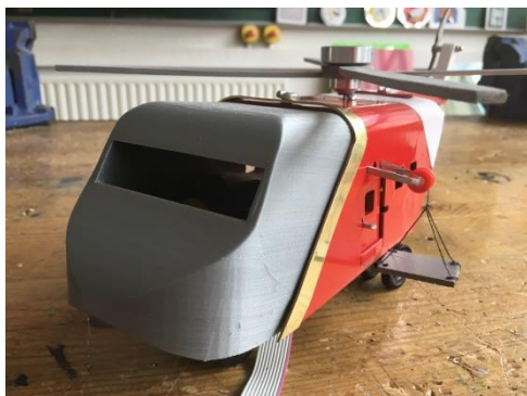
The finished component attached to the final project. The component was a close fit on the fuselage
