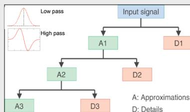
Fig. 2: Convolving the image with high and low pass filters yields details at each level for N levels of decomposition.
