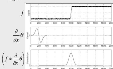
Fig. 3: The convolution of a DoG to identify an edge in a 1D signal.
