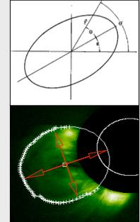
Fig. 6: The inclined ellipse (top) and ellipse fit (bottom) applied to a CME front seen in SECCHI/A onboard STEREO.
