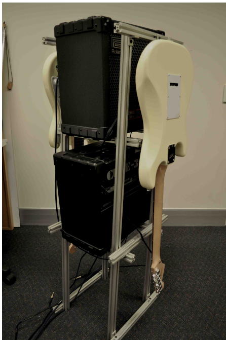
Figure 3: The metal frame used for mounting the electric guitar and amplifier. A second guitar and amplifier system is mounted behind the first, but is not used in this study.
