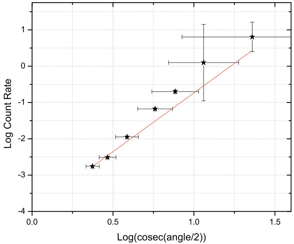
Figure 4: Graph of log Count Rate vs  $\log \operatorname{cosec} \frac{\theta}{2} - y = (3.24 \pm 0.01)x - (3.98 \pm 0.01)$
