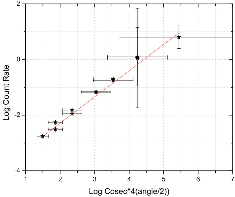
Figure 3: Graph of log Count Rate vs  $\log \operatorname{cosec}^4 \frac{\theta}{2} - y = (0.94 \pm 0.01) - (4.16 \pm 0.01)$
