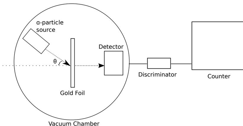
Figure 1: Apparatus of Experiment
