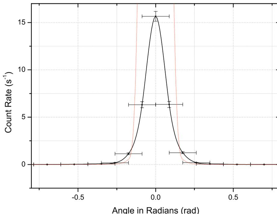
Figure 2: Graph of Count Rate vs Scattering Angle with  $\text{cosec}^4$  normalised to the data
