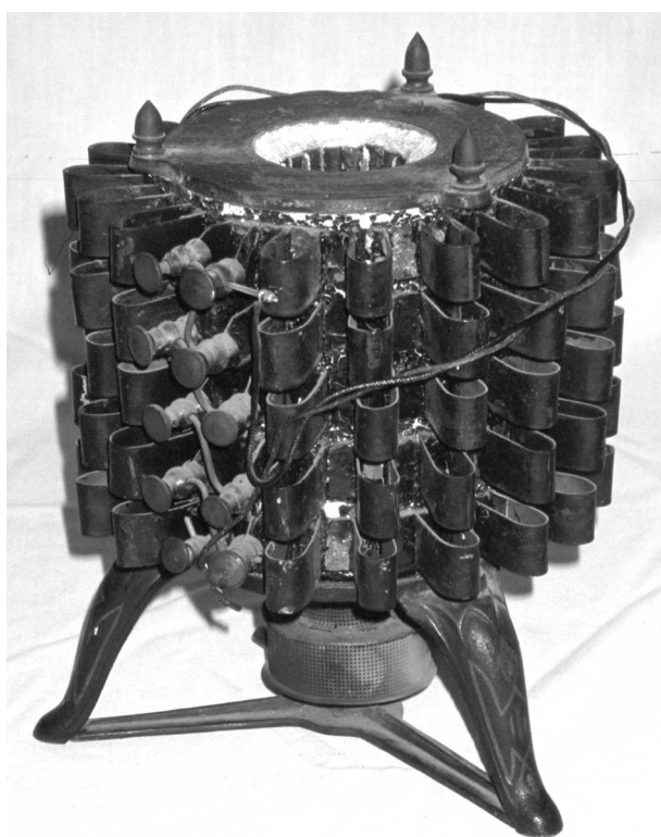
Thermoelectric Battery. At about the turn of the twentieth century, thermoelectric batteries were used to charge storage batteries. The circuit consists of a number of copper and bismuth wires, connected in series. All the copper-to-bismuth connections (for example) are gathered together and kept at one temperature, and the bismuth-to-copper junctions were kept at the other temperature. A gas burner placed in the center of the apparatus raises the temperature of the junctions collected at that point and the other junctions are kept cooler through the use of radiating fins. The overall EMF depends on the number of junctions. This piece of apparatus is at the physics department of Hobart and William Smith Colleges in Geneva, New York. (Photograph and notes by Thomas B. Greenslade, Jr., Kenyon College)
