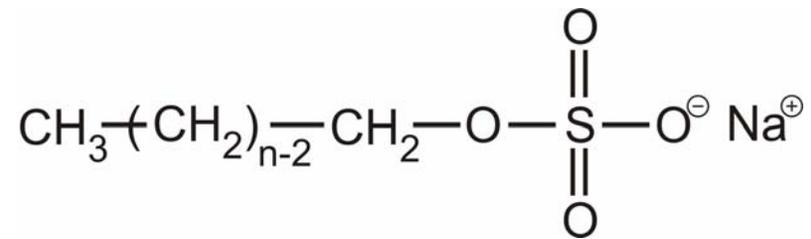
$n=12 \Rightarrow$  sodium dodecyl sulfate, SDS
