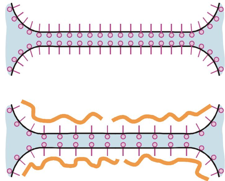
**The spread oil ruptures the thin foam films
