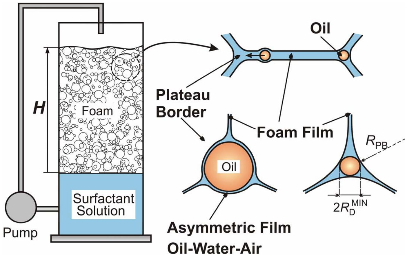
**Key factors: (1) Critical pressure for drop entry (entry barrier)
