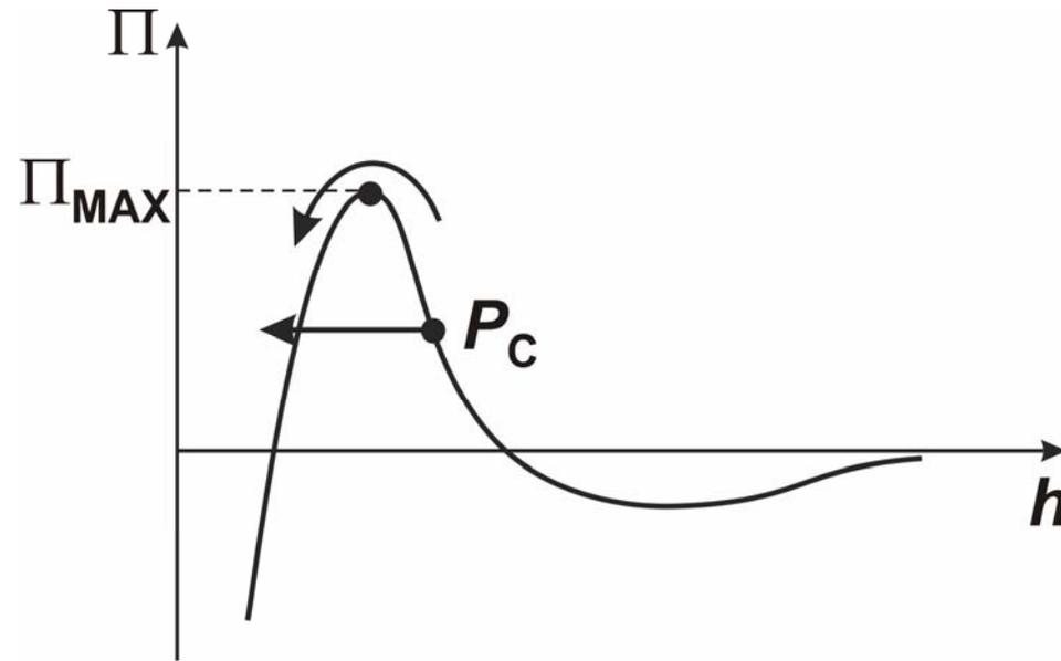
**“Barrier” mode of rupture**
