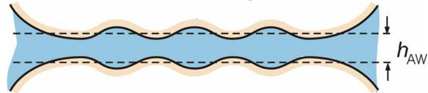
(b) Rupture of thin foam films (surfactant displacement by oil)
