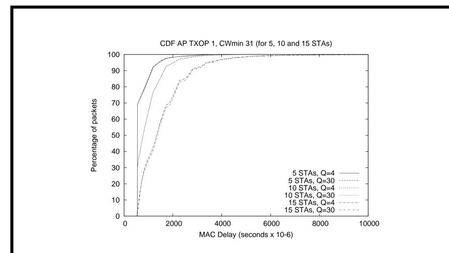
Figure 5: Cumulative distribution for delays at the access point when there are 5, 10 and 15 stations with standard MAC settings.
