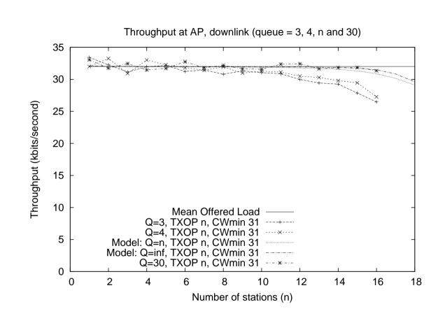
Figure 7: Throughput at the AP for prioritised voice, with TXOP = n packets.
