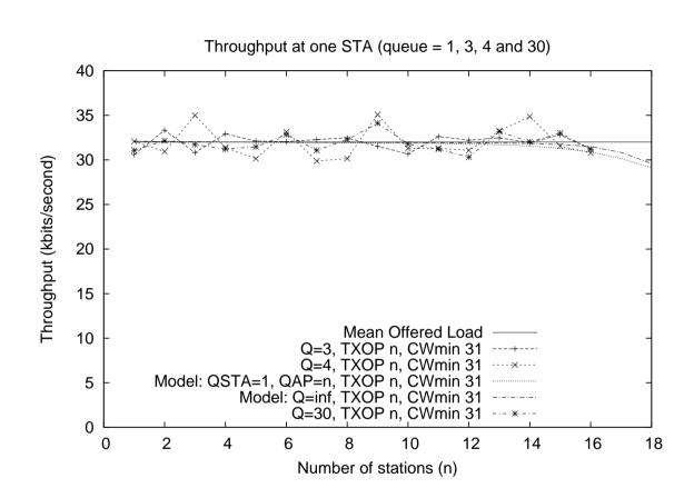
Figure 9: Throughput at a STA for prioritised voice, with TXOP = n packets at the AP.
