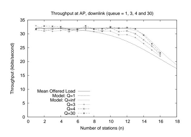
Figure 1: Measured and modelled throughput at the AP. Buffer size at the AP and the STAs is the same. Analytic model also shown.
