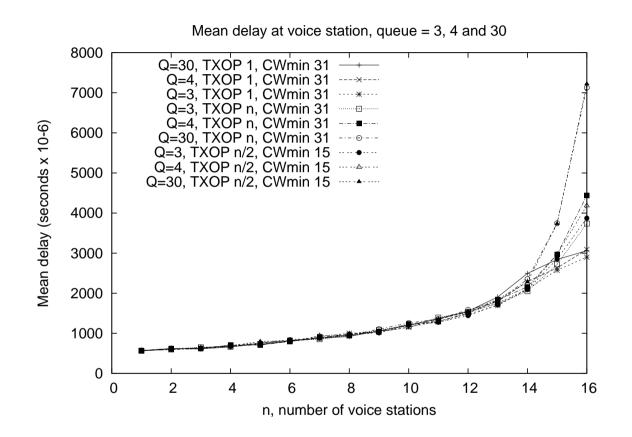
Figure 11: Mean MAC delay a station. The mean interpacket arrival time at a STA is  $10000\mu s$ .
