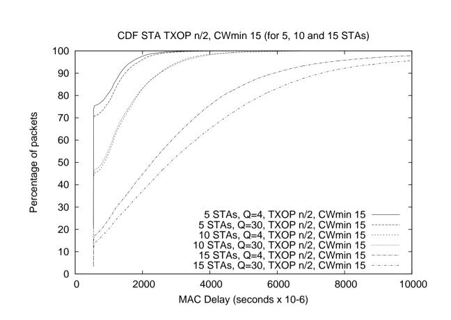
Figure 15: Cumulative distribution for delays at a station when there are 5, 10 and 15 stations when the AP is prioritised using TXOP = n/2 and  $CW_{min} = 15$ .
