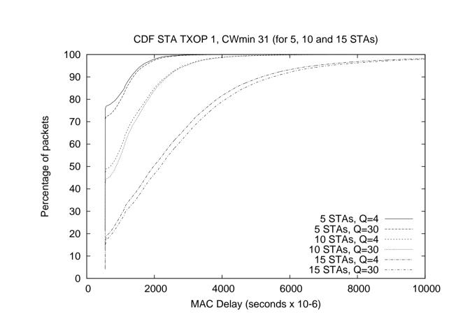
Figure 6: Cumulative distribution for delays at a station when there are 5, 10 and 15 stations with standard MAC settings.
