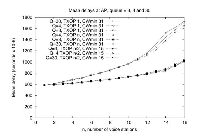
Figure 10: Mean MAC delay at the AP. The group with longer mean delays correspond to the experiments in which the AP is not prioritised.
