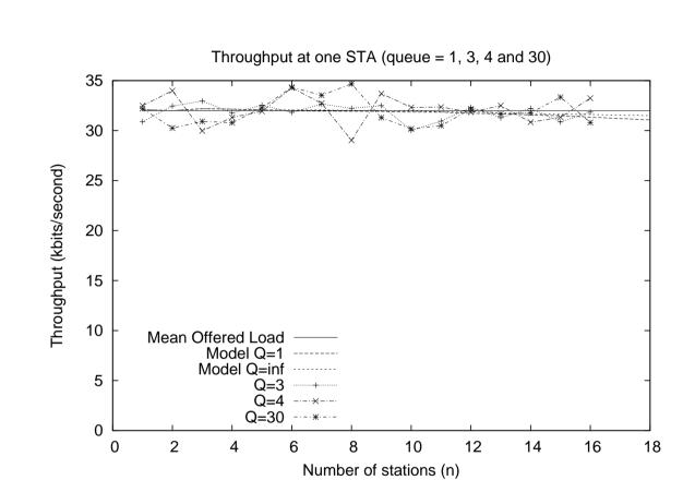
Figure 2: Measured and modelled throughput at a single STA. The buffer size at the AP and the STAs is the same.
