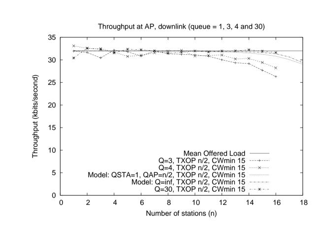
Figure 8: Throughput at the AP for prioritised voice,  $TXOP = n/2, CW_{min} = 15.$
