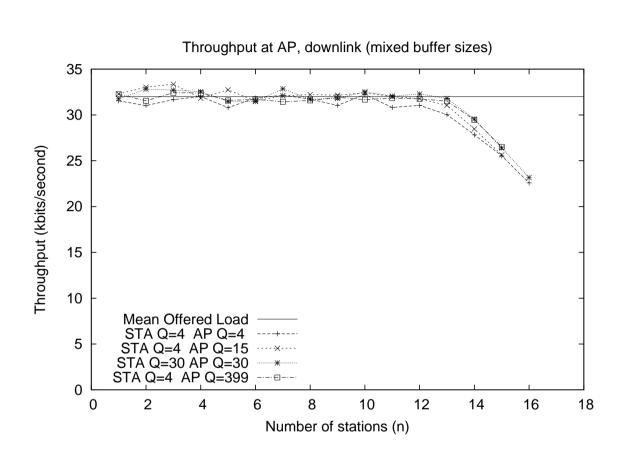
Figure 3: Measured throughput at the AP. Results are shown for various combinations of buffer sizes at the STAs and the AP.
