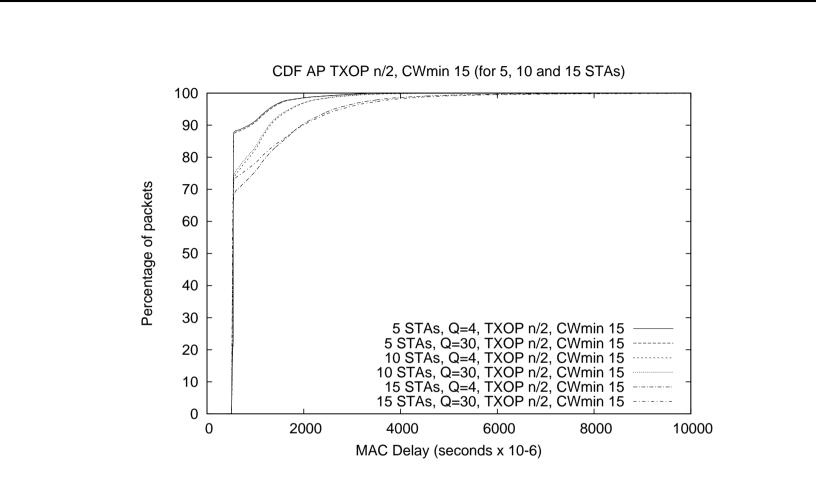
Figure 12: Cumulative distribution for delays at the AP when there are 5, 10 and 15 stations and the AP is prioritised using TXOP = n/2 and  $CW_{min} = 15$ .
