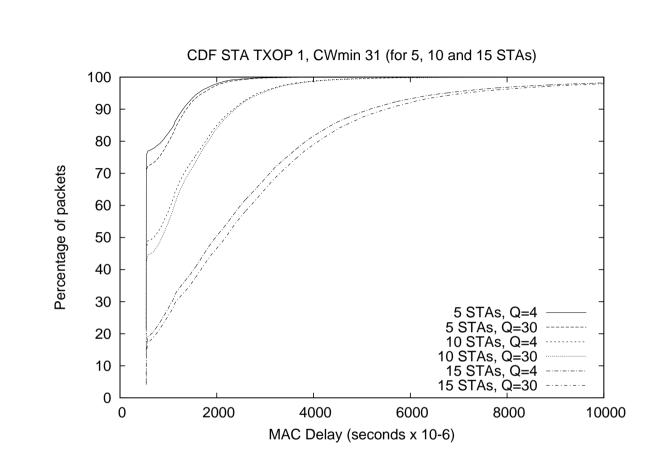
Figure 13: Cumulative distribution for delays at a station when there are 5, 10 and 15 stations with standard MAC settings.
