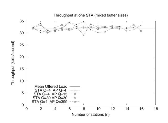
Figure 4: Measured throughput at a single STA. Results are shown for various combinations of buffer sizes at the STAs and the AP.
