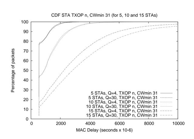
Figure 14: Cumulative distribution for delays at a station when there are 5, 10 and 15 stations and the AP is prioritised using TXOP = n.
