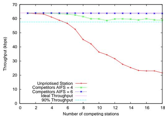
Fig. 6. Throughput by a voice call competing with saturated stations.
