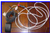
GPS unit with cigarette lighter attachment and serial port
