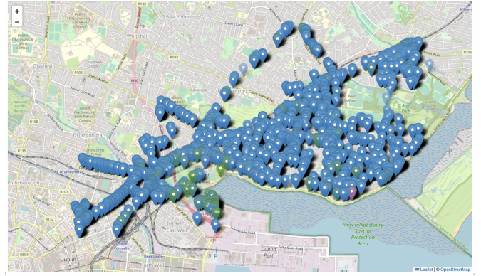
Fig. 2. Networks detected in the Clontarf area in 2002 (left) and 2022 (right). Green denotes unencrypted networks, red denotes networks using WEP and blue denotes networks using WPA/WPA2.
