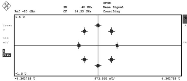
Fig 6. Demodulated constellation of the physical layer decrypted 8PSK signal captured on R&S FSQ at 14.23 GHz
