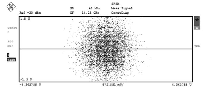
Fig 5. Demodulated constellation of the physical layer encrypted 8PSK signal captured on R&S FSQ at 14.23 GHz
