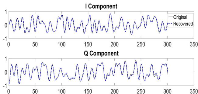
Fig. 8 Comparison of the demodulated baseband I and Q waveforms from the original carrier and from the encrypted carrier after recovery with the decryption filter.
