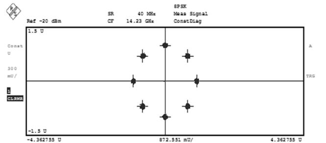
Fig 4. Demodulated constellation of the original 8PSK signal captured on R&S FSQ at 14.23 GHz
