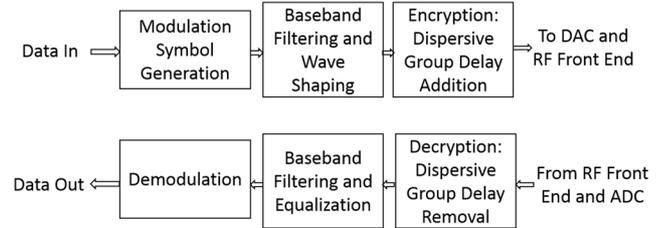
Fig 3 Proposed Physical Layer Encryption Scheme
