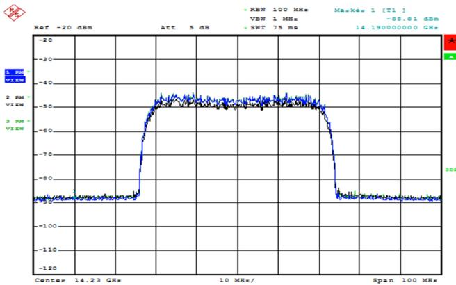
Fig 7. Power spectrum comparison screenshot captured on R&S FSQ at 14.23 GHz. Trace 1 (black): Original 8PSK carrier, Trace 2 (blue): Encrypted 8PSK carrier, Trace 3 (green): Decrypted 8PSK carrier
