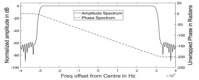
Fig 2 Spectral characteristics of a digital FIR filter.
