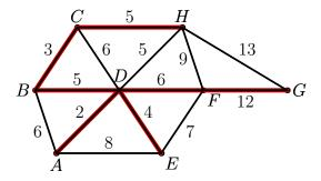
The minimal spanning tree generated by Kruskal's Algorithm thus consists of the vertices A, B, C, D, E, F G and H of the given connected graph, together with the edges  $e_1$ ,  $e_2$ ,  $e_3$ ,  $e_4$ ,  $e_5$ ,  $e_6$  and  $e_7$ , where  $e_1, \ldots, e_7$  denote the edges of the minimal spanning tree listed in the order in which they were added to the acyclic graph, so that
