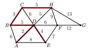
Adding the edge *DH* would create a circuit *DBCHD*; therefore the edge *DH* is discarded. Adding the edge *AB* would create a circuit *ABDA*; therefore the edge *AB* is discarded. Adding the edge *CD* would create a circuit *DBCD*; therefore the edge *CD* is discarded.
