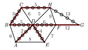
The spanning tree T' includes edges  $e_i$  of the Kruskal spanning tree for i < 7 but does not include the edge  $e_7$ , where  $e_7 = FG$ . Now addition of the edge  $e_7$  to the spanning tree creates a circuit *FGHCBDF* in the resultant subgraph. This circuit cannot consist entirely of edges of the Kruskal tree. Therefore at least one edge of the circuit does not belong to the Kruskal tree. That edge is *GH*.
