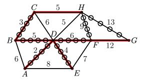
Adding any edge to a spanning tree creates a circuit. In particular, if we add the edge CH to the spanning tree T, then the resultant subgraph of the original connected graph must contain a circuit. In the present example the circuit created is CHFDBC. Now not all edges of that circuit can belong to the Kruskal tree, because trees cannot contain circuits. Therefore at least one edge of the circuit CHFDBC does not belong to the Kruskal tree.
