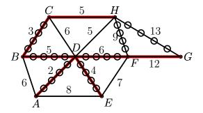
It follows that we can modify the spanning tree T to obtain a new spanning tree T', where T' includes the edges  $e_1$ ,  $e_2$ ,  $e_3$ ,  $e_4$  and  $e_5$  of the Kruskal tree, and where the cost of T' does not exceed that of T. The resultant tree T' consists of the edges with circles in the following figure:—
