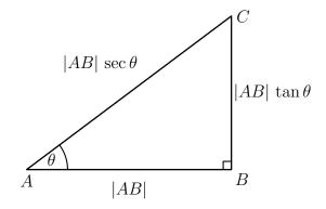
In the above triangle ABC, in which the angle at the vertex B is a right angle, the lengths |AC|, |AB| and |BC| satisfy the identities
