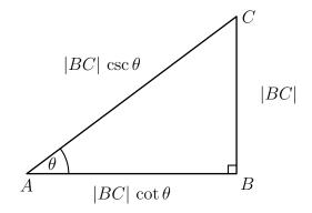
In the above triangle ABC, in which the angle at the vertex B is a right angle, the lengths |AC|, |AB| and |BC| satisfy the identities
