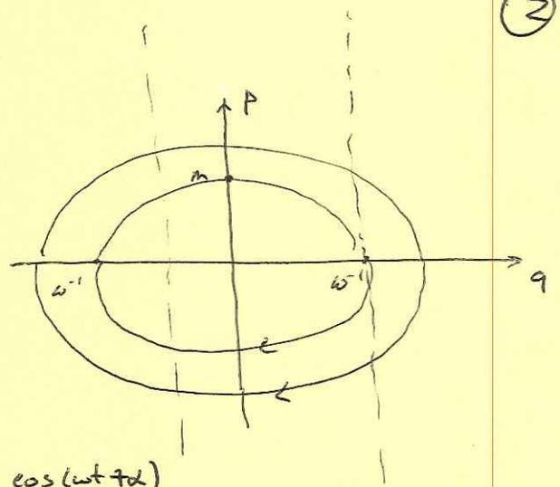
$$p = \cos(\omega t) p_i - \sin(\omega t) m \omega q_i = m A \cos(\omega t + \alpha)$$
