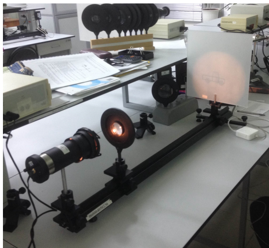
Figure 2: The apparatus consists of an optical rail with supports, an incandescent electric lamp, a translucent screen, and various converging and diverging lenses.
