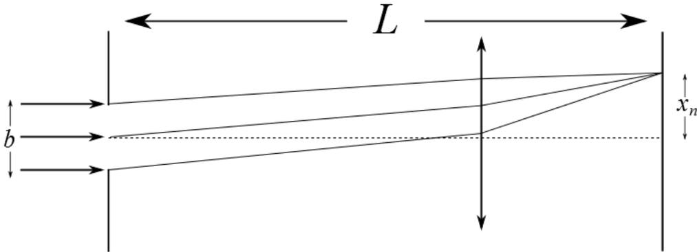
Figure 1: Fraunhofer diffraction at a slit.
