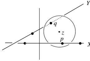
Figure 2: Sphere tangent to two lines at two given points.
