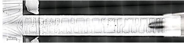
Figure 3. Exemplary SU-8 micro-beam glued to a glass support (on the left hand side) and loaded with a single force by the AFM Tip (on the right hand side). Recorded by optical microscopy.
