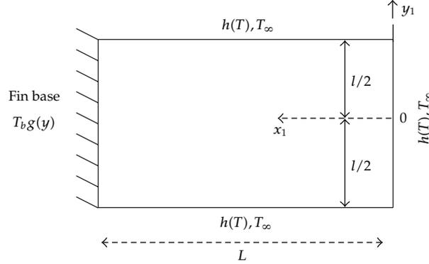
**Figure 1:** Schematic representation of a rectangular straight fin.
