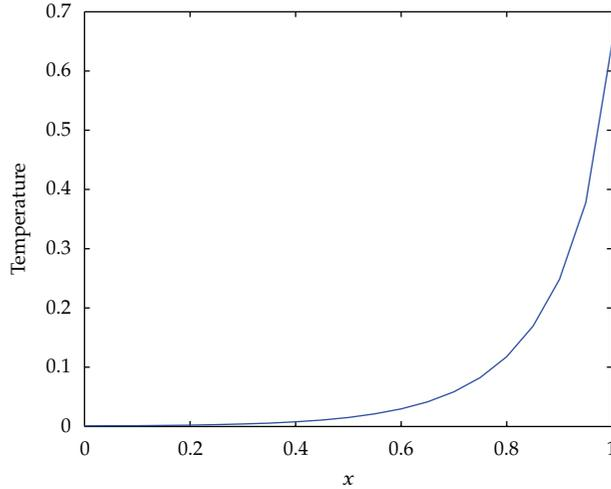
(a) Temperature profile at  $y = 1$ . Parameters used are  $Bi_\phi = Bi_\psi = 0.02$ ,  $E = 2$
