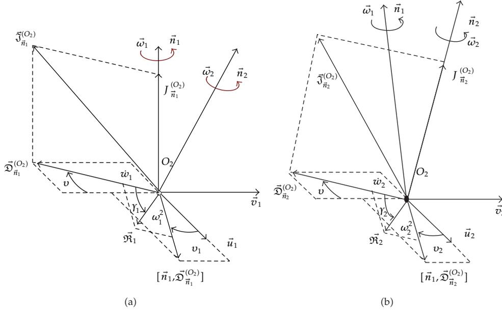
**Figure 2:** Vector rotators  $\vec{\mathfrak{R}}_1$  (a) and  $\vec{\mathfrak{R}}_2$  (b) in relations to corresponding mass moment vectors  $\vec{J}_{\vec{n}_1}^{(O_2)}$  and  $\vec{J}_{\vec{n}_2}^{(O_2)}$ , and their corresponding deviational components  $\vec{\mathfrak{D}}_{\vec{n}_1}^{(O_2)}$  and  $\vec{\mathfrak{D}}_{\vec{n}_2}^{(O_2)}$  as well as to corresponding deviational planes.
