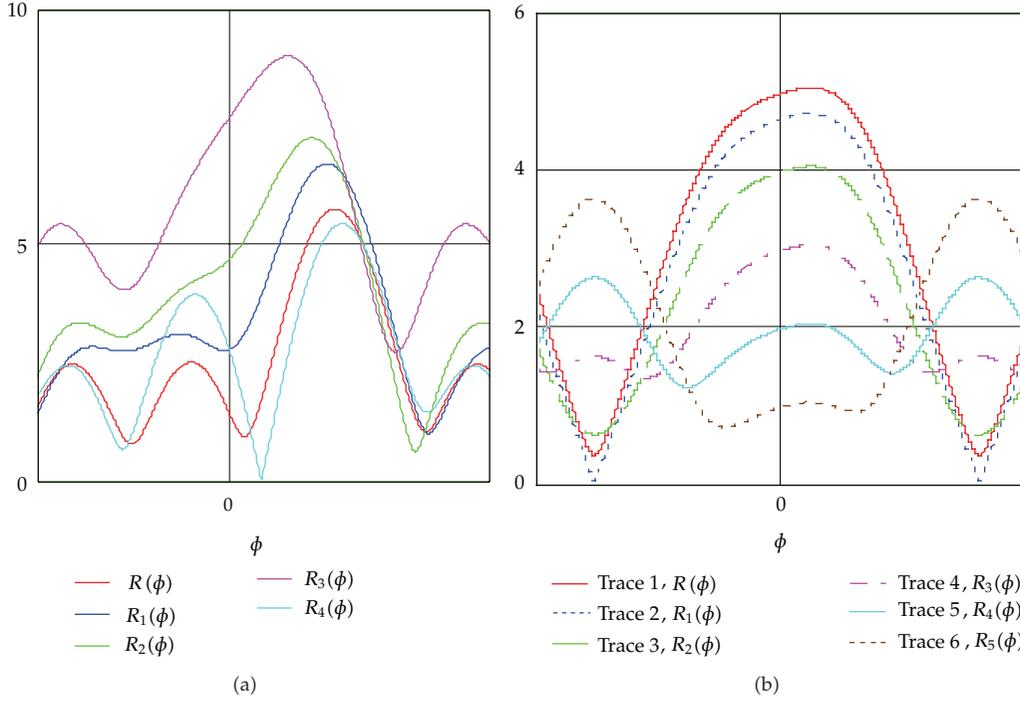
**Figure 5:** Intensity of vector rotators  $\vec{\mathfrak{R}}_{022}$  and  $\vec{\mathfrak{R}}_2$ , for different disk eccentricity (a) and for different initial conditions (b).
