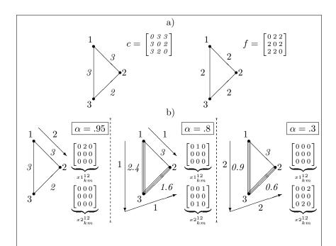
Figure 1. a) An example of a network with specified costs c and flow demands f; b) Sending 2 units of flow from origin 1 to destination 2, depending on three different values of  $\alpha$ . Threshold is T=3.
