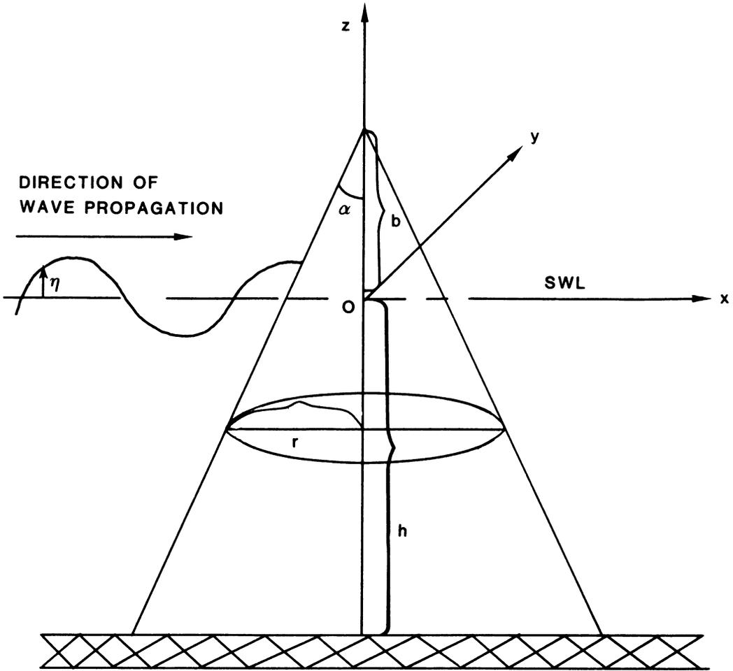
**FIG.7. Schematic Diagram of a Conical Structure in waves.**
