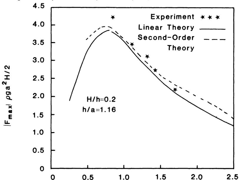
FIG. 6. Comparison of linear and second-order wave forces with experimental data of Chakrabarti [13].
