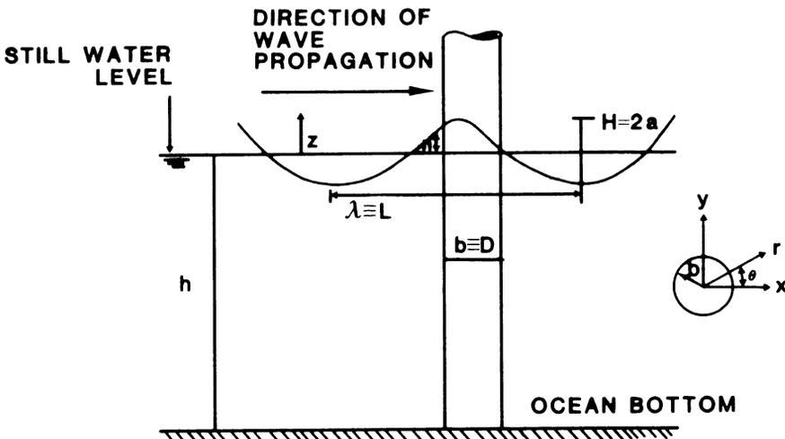
**FIG. 1. Schematic diagram of a cylindrical structure in waves**
