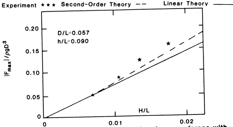
FIG. 2. Comparison of linear and second-order wave forces with experimental data of Mogridge and Jamieson [3].
