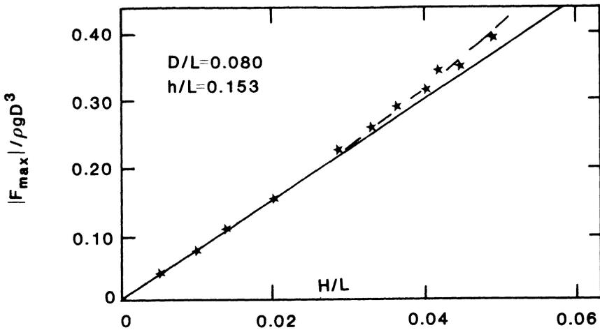
FIG. 4 Comparison of linear and second-order wave forces with experimental data of Mogridge and Jamieson [3].
