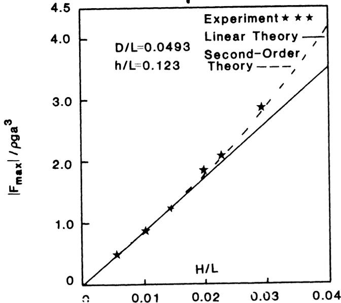
FIG. 5. Comparison of linear and second-order wave forces with experimental data of Raman and Venkatanarasaiah [24].
