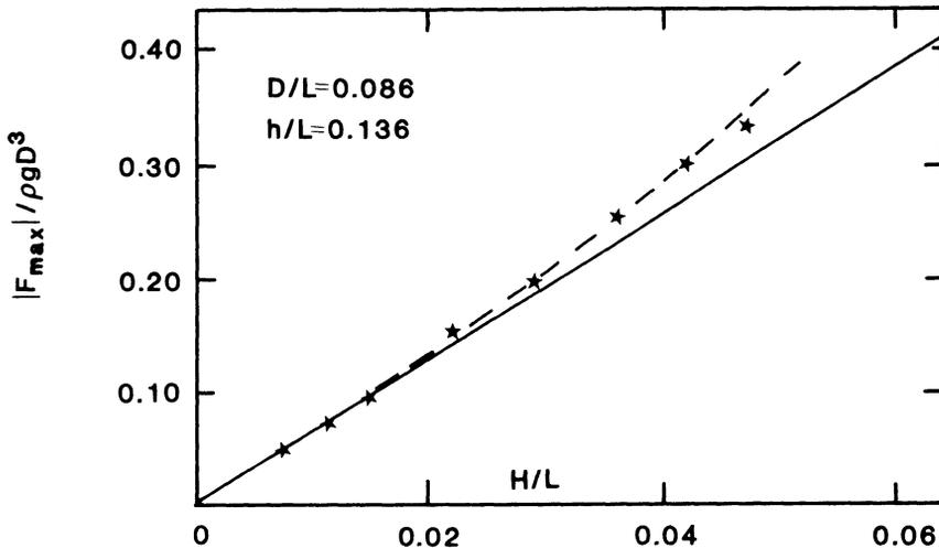
FIG. 3. Comparison of linear and second-order wave forces with experimental data of Mogridge and Jamieson [3].
