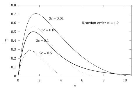
FIGURE 5.7. Velocity profiles for n = 1.2.
