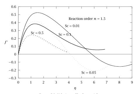
Figure 5.9. Velocity profiles for n = 1.5.
