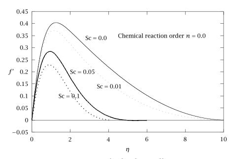
FIGURE 5.5. Zeroth order velocity profiles.
