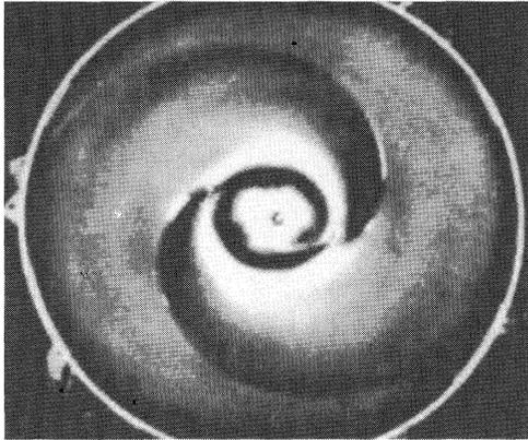
FIGURE 15 Trailing spiral waves of surface density excited in differentially rotating shallow water: mode  $m=2$  with  $\Omega_1=13$  rad/s,  $\Omega_2=2.6$  rad/s, shallow water thickness  $H=0.35$  cm. The core, the periphery, and the spiral pattern are rotating clockwise. The angular velocity of the pattern rotation is  $\Omega_p=6$  rad/s. The dark circle intersected by the spiral arms is the line of the rotation velocity jump.
