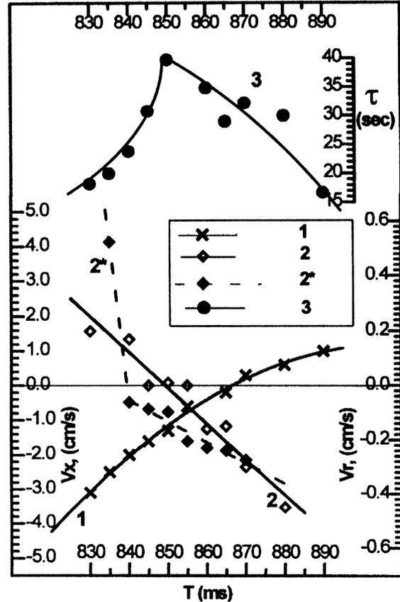
FIGURE 4 Drift velocities of the Rossby anticyclones: along the  $X$ -axis ( $V_x$ , 1) and in radial direction ( $V_r$ , 2) and the vortex life times  $t$  (3) as functions of the paraboloid rotation period,  $T$ . The vortex amplitude  $h \cong 0.1$ . Dependence  $V_r(T)$  for a large vortex amplitude ( $h \cong +1.1$ ) is shown by the curve 2\*. In the latter case the nonlinearity eliminates the meridional vortex drift (and even changes its direction) in a definite region of  $T$ .
