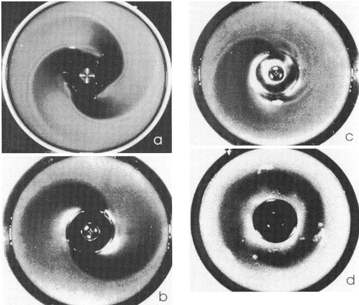
FIGURE 14 (a)–(d): Trailing spiral waves of surface density excited in differentially rotating shallow water: azimuthal modes  $m=3, 2, 1, 0$ . The “core” and the spiral pattern are rotating clockwise, the “periphery” is at rest. Black (white) parts of the pattern are the elevations (depressions) of the shallow water.
