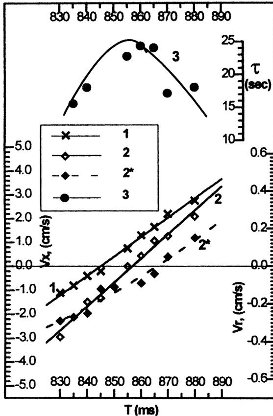
FIGURE 3 Drift velocities of the Rossby cyclones: along the  $X$ -axis ( $V_x$ , 1) and in radial direction ( $V_r$ , 2) and the vortex life times  $t$  (3) as functions of the paraboloid rotation period,  $T$ . The vortex amplitude  $h \cong -0.1$ . Dependence  $V_r(T)$  for a large vortex amplitude ( $h \cong -0.3$ ) is shown by the curve 2\*. In the latter case the nonlinearity eliminates the meridional vortex drift (and even changes its direction) in a definite region of  $T$ .
