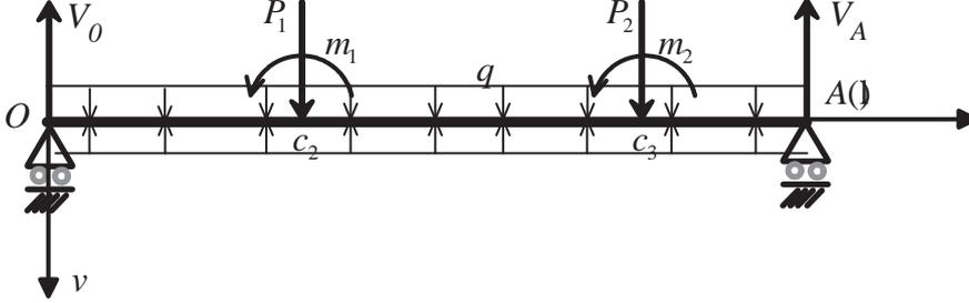
Fig. 1. Elastic rod supported on an elastic foundation
