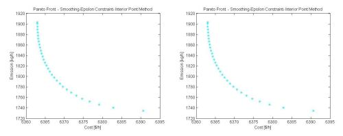
Figure 2: Pareto Front using Smoothing- $\epsilon$ -constraint - Interior point method for  $\mu=0.000001$ .
