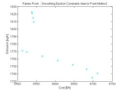
Figure 6: Pareto Front using Smoothing- $\epsilon$ -constraint - Interior point method for  $\mu=0.5$ .
