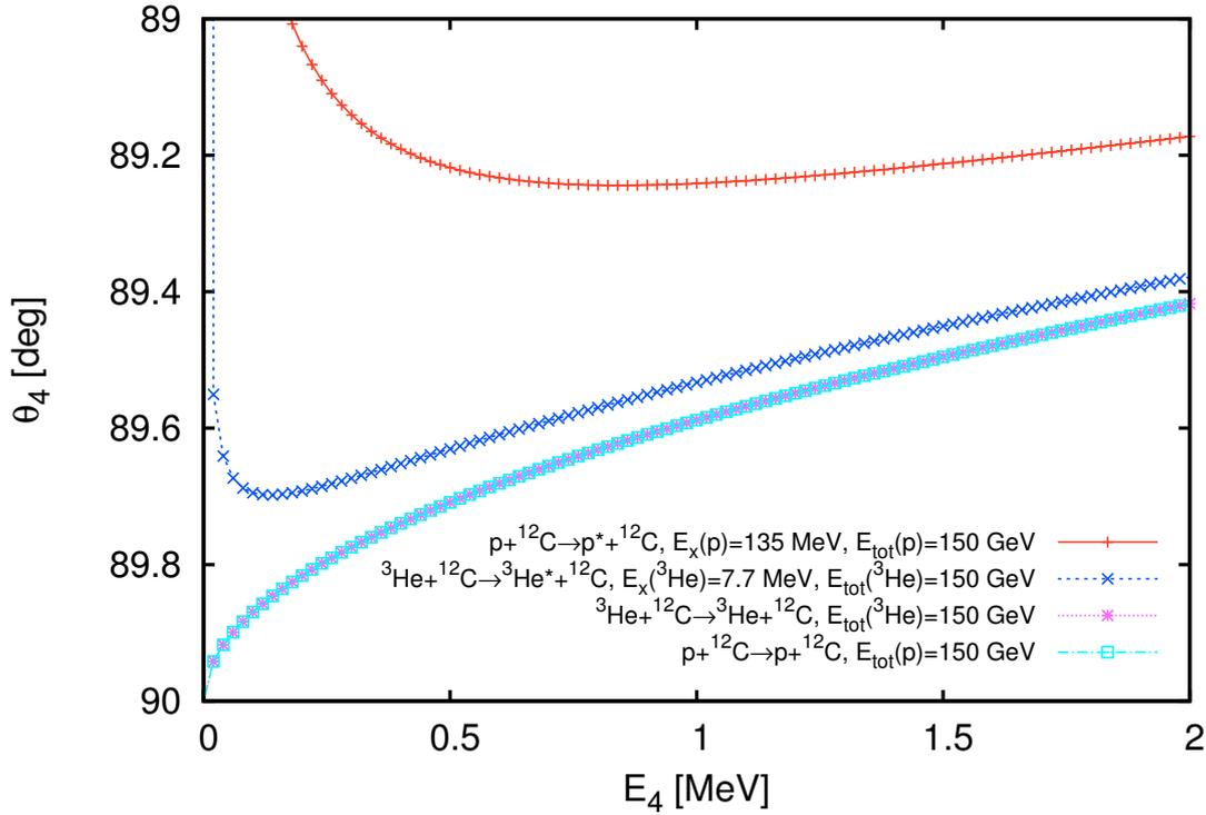
**Figure 2:** The laboratory angle  $\theta_4$  of a recoiling carbon nucleus versus its recoil kinetic energy  $E_4$  for (from top) (1) a 150 GeV proton scattering to  $p\pi^0$ , (2) a helion of energy 50 GeV/nucleon scattering to break-up, (3) a helion of energy 50 GeV/nucleon scattering elastically, (4) a 150 GeV proton scattering elastically. Curves for the elastic scattering of helions and protons with the same energies are almost indistinguishable.
