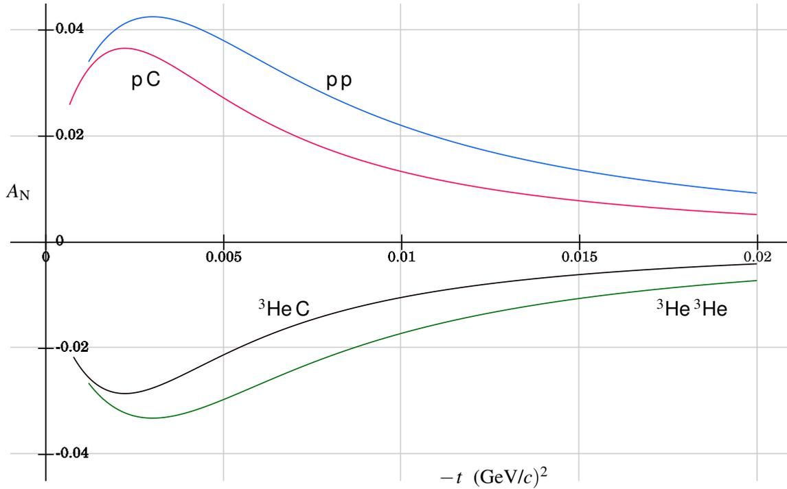
**Figure 1:** Analyzing power  $A_N$  versus the squared momentum transfer variable  $(-t)$  for the elastic scattering processes (from the top): (1) proton proton, (2) proton carbon, (3) helium-3 carbon, (4) helium-3 helium-3, assuming that  $\sigma_{\text{tot}}(\text{hC}) = 2\sigma_{\text{tot}}(\text{pC})$ , that  $\sigma_{\text{tot}}(\text{hh}) = 4\sigma_{\text{tot}}(\text{pp})$ , and that  $\rho$ ,  $\delta$ ,  $R_S$ ,  $I_S$ , and finite nuclear size effects are negligible.
