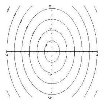
The trajectories go anticlockwise because the sine part is negative and the cosine part positive, think what happens for small t,  $y_1$  is still pretty close to r and  $y_2$  is negative.
