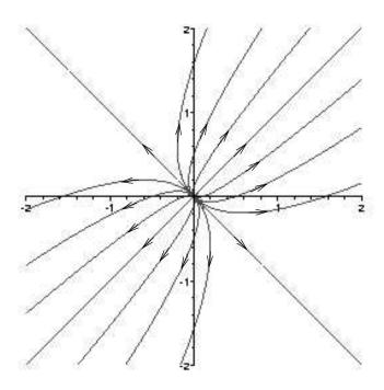
As with the proper node, it could also happen that the two eigenvalues are negative, in which case the arrows would point inward rather than outward. A long way from the origin, the trajectories bend so that they are parallel to the larger, in the sense of more negative, of the two eigenvalues. The way to think about this is to ask, for a given  $c_1$  and  $c_2$  where did the trajectory come from, in other words what happens for large negative t. Thus, if  $\lambda_1 = -4$  with
