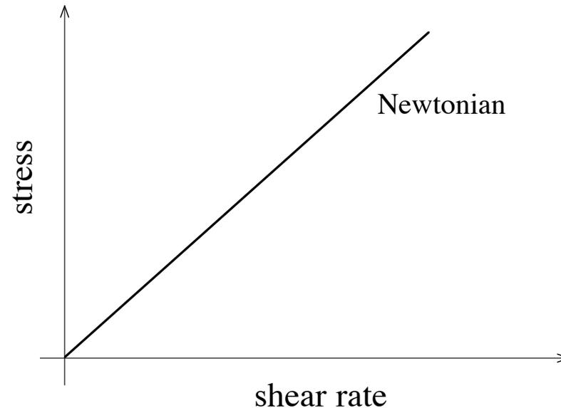
Newtonian case is linear, slope is the viscosity  $\eta$
