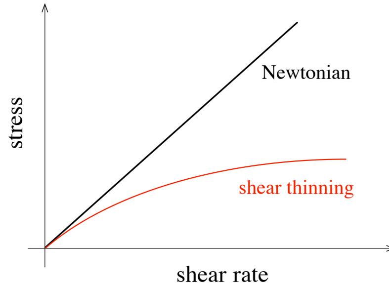
More complex, structured fluids can be nonlinear in shear.
