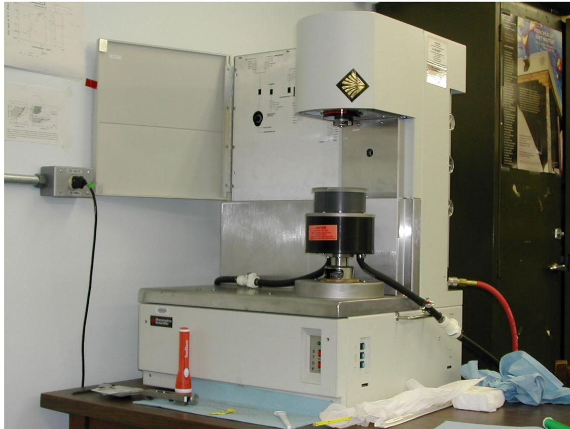
Rheometrics (TA Inst) RFS-III controlled rate of strain rheometer
