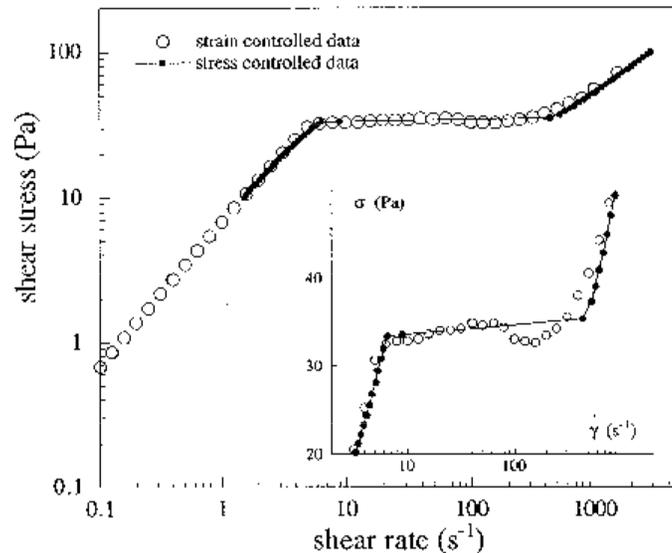
FIG. 4. Comparison between the  $\sigma(\dot{\gamma})$  values in a log-log representation obtained with a controlled shear rate (open symbols) and a controlled shear stress (closed symbols) rheometer for the CTAB-D<sub>2</sub>O without salt system at  $T=32$  °C. Shown in the inset is the variation of the shear stress versus shear rate in a semilogarithmic representation.
