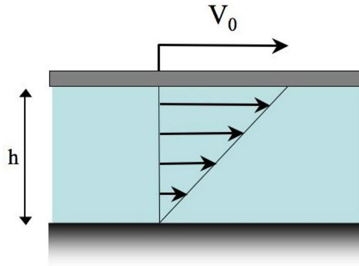
For certain materials the force per unit area  $\sigma$  on the moving plate will be proportional to  $V_0$ , and inversely proportional to  $h$ :
