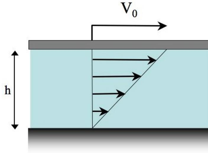
In this simple geometry the velocity field will be linearly dependent on the distance  $y$  from the stationary plate:
