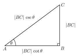
In the above triangle ABC, in which the angle at the vertex B is a right angle, the lengths |AC|, |AB| and |BC| satisfy the identities
