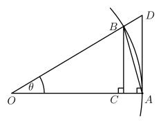
The sector OAB of the unit circle is by definition the region bounded by the arc AB of the circle and the radii OA and OB. Now the area of a sector of a circle subtending at the centre an angle of  $\theta$  radians is equal to the area of the circle multiplied by  $\frac{\theta}{2\pi}$ . But the area of a circle of unit radius is  $\pi$ . It follows that a sector of the unit circle subtending at the centre an angle of  $\theta$  radians has area  $\frac{1}{2}\theta$ .
